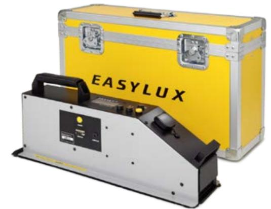
**EasyLux Horizontal classic for road markings** is robust, simple and intuitive handling instrument which can simultaneously evaluate 30-meter (or 15-meter) nighttime visibility  $R_L$ , daytime visibility  $Q_d$  and register the ambient temperature and relative air humidity quickly, easily and effortlessly. Complies with ASTM E1710, ASTM E2302, ASTM E2177, EN1436.
