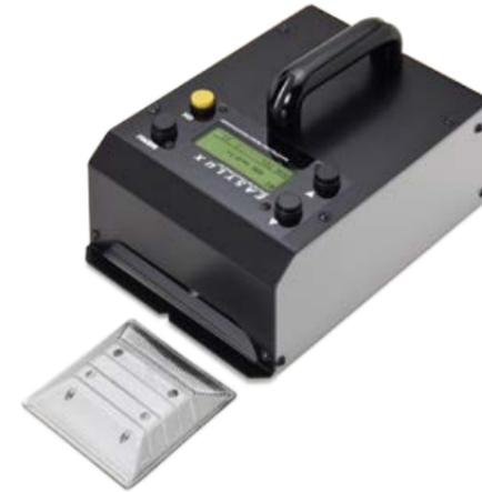
**EasyLux Road Studs retroreflectorometer** is a robust and very compact instrument. Weighing only 3 kg it was designed to measure the retroreflection  $R_I$  of all types and colors of road studs. Complies with ASTM E1696, EN1463.
