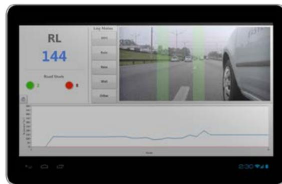
**Dynamic retroreflectometer** wireless remote tablet:
